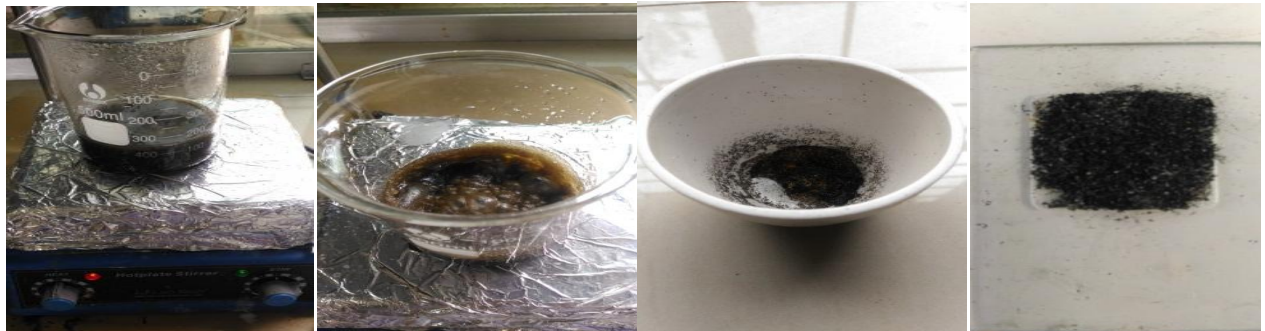
Figure 1 Photograph of preparation of graphenic material coated sand composite GSC
