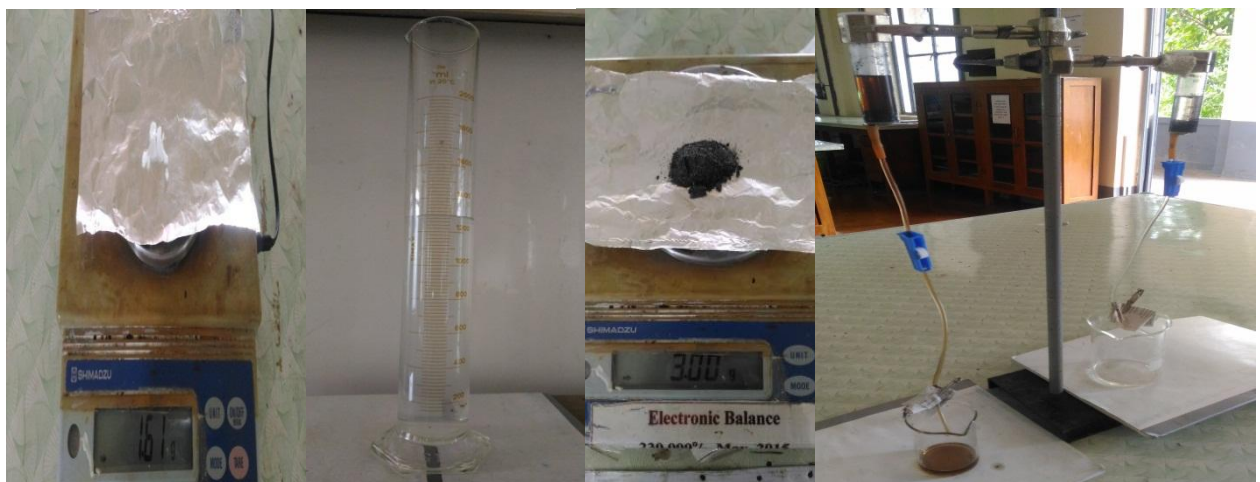
Figure 2 Photograph of preparation of Pb 2+ solution and Filtration with GSC.
